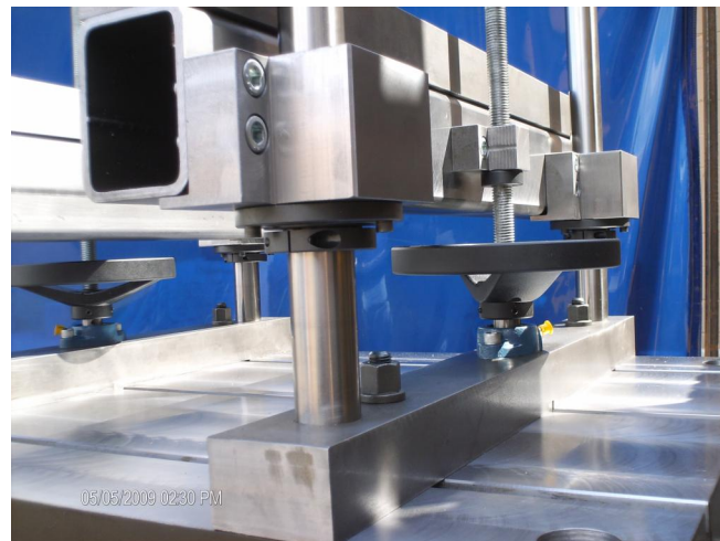
X-Y-Z positioner unit with 7-pillar guide for the mounting of a driving unit
