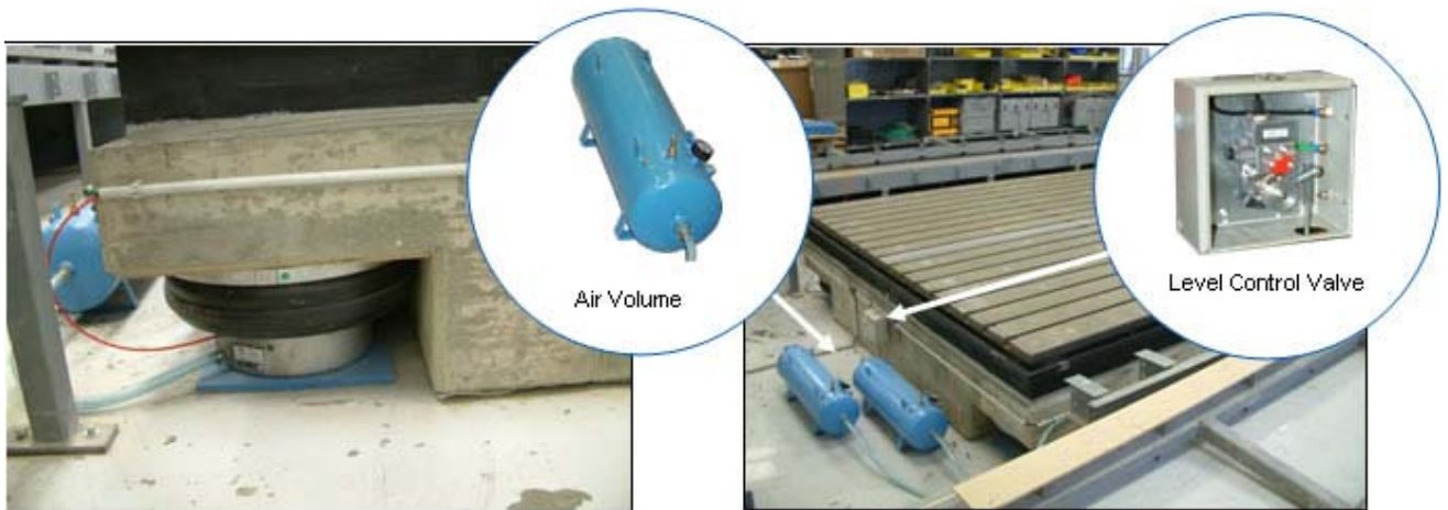
Air Spring GRB with additional air volume attached for reduction of the 1 st natural frequency from 1.2 Hz to 0.8 Hz. View on one of the three level control valves attached to the side wall of the seismic mass.
