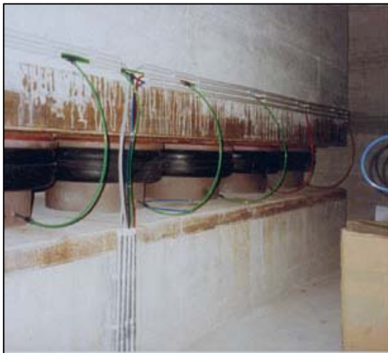
600 to Seismic mass on CFM-Schiller GRB air springs. Natural frequency approx. 1.2 Hz
