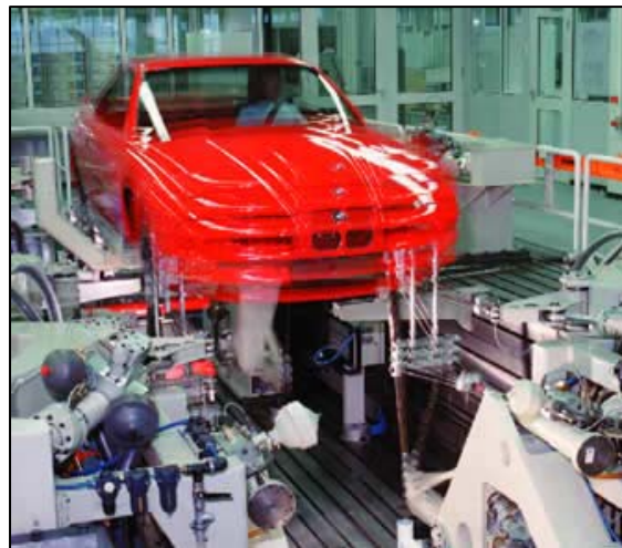
Isolated seismic mass with floor plate and dynamic test equipment acting on a car body.
