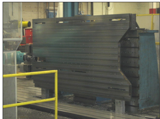
6 Custom Steel base plates for an X-Y positioning system manufactured for Porsche, Germany
