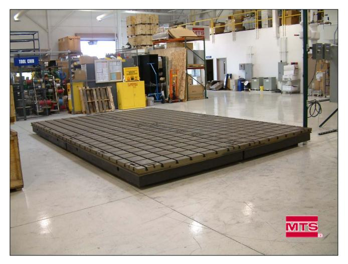
Base plate with crossed T-slots, joints and caps sealed. Can be re-arranged in many different configurations (T-shape, 2 separate fields etc). Plate mounted on rubber vibration isolators with 1<sup>st</sup> natural frequency around 7 Hz. Protective wax still applied to the plate surfaces.
