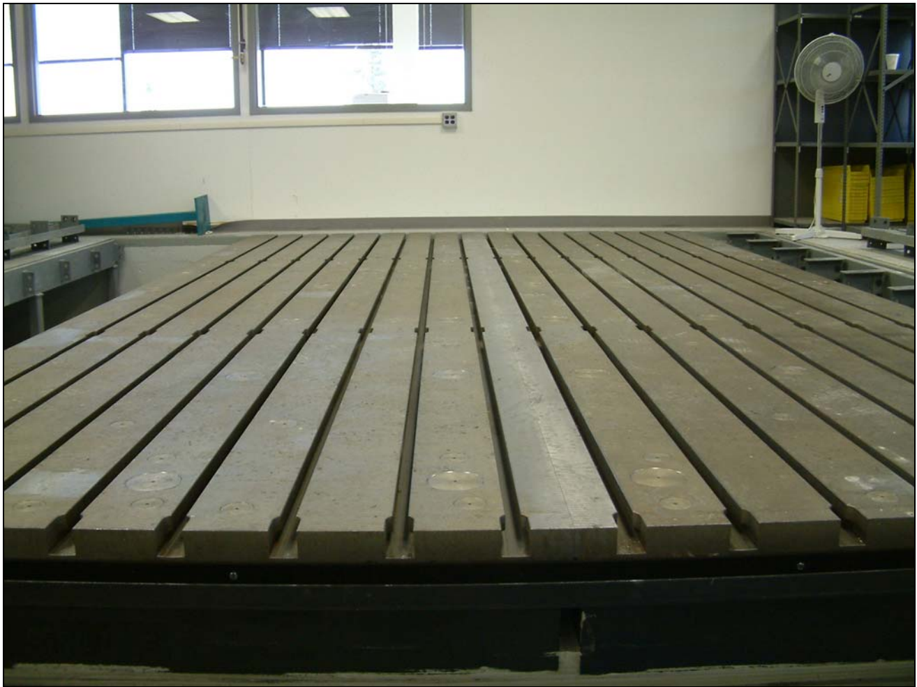
Base plate 6000 x 3440 x 350 mm with protective wax cover
