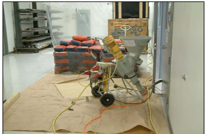
Grout Pump "PABEC III" for continuous pumping of the grout for up to 5 to/hour.
